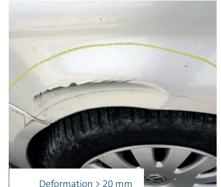
Deformation &gt; 20 mm
