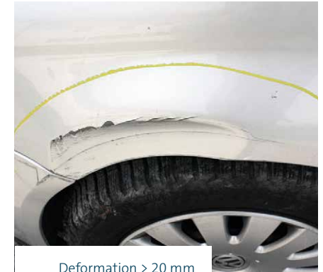
Deformation &gt; 20 mm
